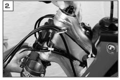
Slide the lower triple clamp into the steering head, holding the upper steering head bearing and the sealing washer in place.
