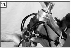
Holding on to the lower triple clamp, remove the adjusting nut on the steering head bearing.
