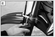
Remove the brake line guide.
