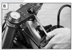
Tighten the collar screw ( 8 ) to clamp the shaft tube to  $20\ \text{Nm}.$
