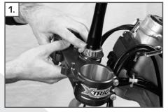
Grease the steering head bearing on the pre-assembled XTRIG triple clamp with suitable bearing grease.
