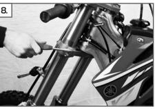
Loosen the triple clamp clampings.
