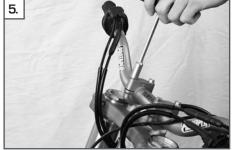
Remove the handlebar and any fastening material such as cable ties.
