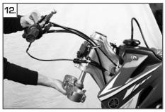
Remove the lower triple clamp. Clean the motorcycle's steering head and bearing seat.
