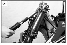
Position the fork, front wheel and brake system in the triple clamp.
