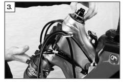
Depending on the model, mount the seal for the steering head bearing (sealing washer or O-ring)
