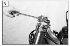
Use the adjusting nut ( 4 ) to adjust the desired bearing clearance.
