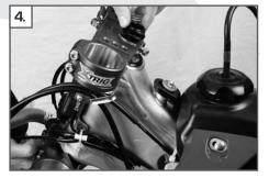
Mount the upper triple clamp and screw the adjusting nut ( 4 ) on by hand.
