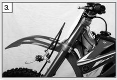
Attach the brake pump to the brake line.
