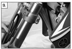
Pull the fork down and remove together with the front wheel and brake system.
