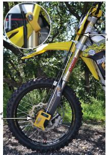
Make sure butt of clip is against plate to avoid rotating.
