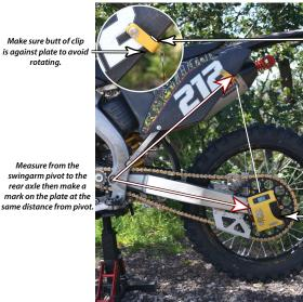
Right edge of clip aligns with mark made on plate.
